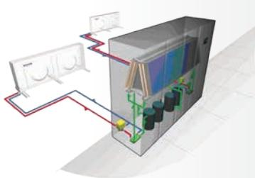
Configuration direct expansion water-cooled with double refrigerant circuit.
