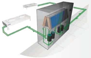
Configuration with air-cooled direct expansion with double refrigerant circuit.
