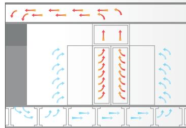
With increasing density of servers, a solution to open aisles may not be sufficient to ensure proper cooling of the rack. In these applications, in fact increases the risk of mixing between the two streams, that can be avoided by closing aisles and confining the air flows. We identify two possible solutions:
