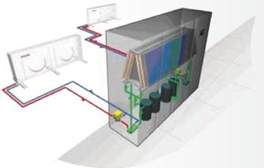
Configuration direct expansion water-cooled with double refrigerant circuit.
