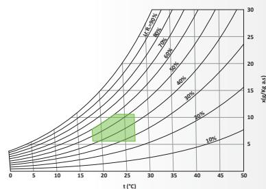
The humidity content, in server rooms, is very important. Too high humidity values can lead to mistakes of tape bearing, excessive wear and corrosion. These risks increase exponentially when the relative humidity exceeds 55%. On the other hand, too low values of relative humidity (below 30%), increase the risk of electrostatic discharge which can damage components and have an adverse effect on the operation of the unit.
