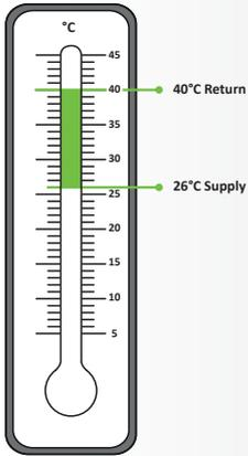
The solution with hot aisle normally includes the supply of air at 21°C and the return at 35°C. A solution with higher working temperatures (27 / 40°C) can lead to an increase in efficiency of the system. The ASHRAE, in fact, in its guidelines for data center design (ASHRAE TC 9.9 – Thermal Guidelines for Data Processing Environments) sets a maximum limit for the supply temperature of 27°C and 40°C for the return.
