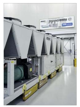
Representing a €5m investment, the new chamber allows units of up to 2.000kW cooling and heating capacities to be tested, and measures 28m in length by 6m in height for a total volume of 2.200m3.
