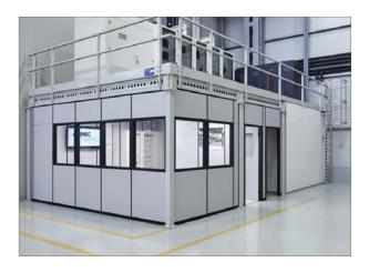
Particular attention has also been afforded to Customer witness testing, an ever increasing requirement for large projects. Then new test labs will feature a dedicated Customer witness room where all parameters can be instantly and graphically monitored and recorded, specific Customer requests can be quickly implemented and unit operation can be visualised from the comfort of your chair.
