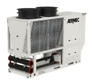
PRM modular reversible heat pump, is built to meet air conditioning needs in residential/commercial complexes or chilling in industrial complexes. It uses R290 natural refrigerant (propane) with ultra-low direct greenhouse effect (GWP = 3) in total safety. Available in one size with nominal heating capacity 100 kW, it can be easily linked in parallel with other identical units to form a hot-cold system serving systems of all sizes.
