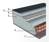
Coeff. of global Transmittance: U= 1,407W/m<sup>2</sup>K
