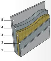
Coeff. of global transmittance: U= 0,671W/m<sup>2</sup>K
