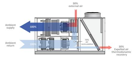
To compare the three system solutions mentioned above, we have considered roof-top systems, whose performances are aligned to the state of the art: the presence of the static recovery with the same percentage of fresh air (30%), useful in keeping the parts of hypothesized fresh air.
