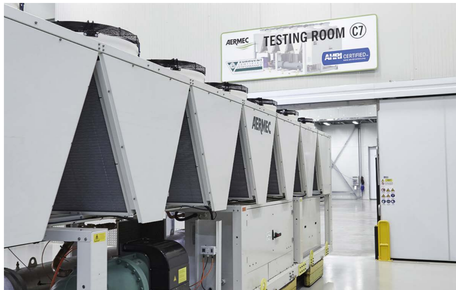
Calorimetric test chamber used to perform Eurovent tests for the certification
